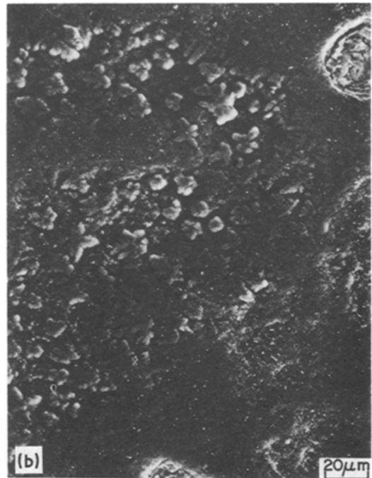
Figure 7 Progressive removal of outer oxidized layer in \text{Si}_3\text{N}_4 oxidized at 1375^\circ\text{C} for 240 h (a) 2.5\ \mu\text{m} removed, (b) 25\ \mu\text{m} removed and (c) 50\ \mu\text{m} removed.
